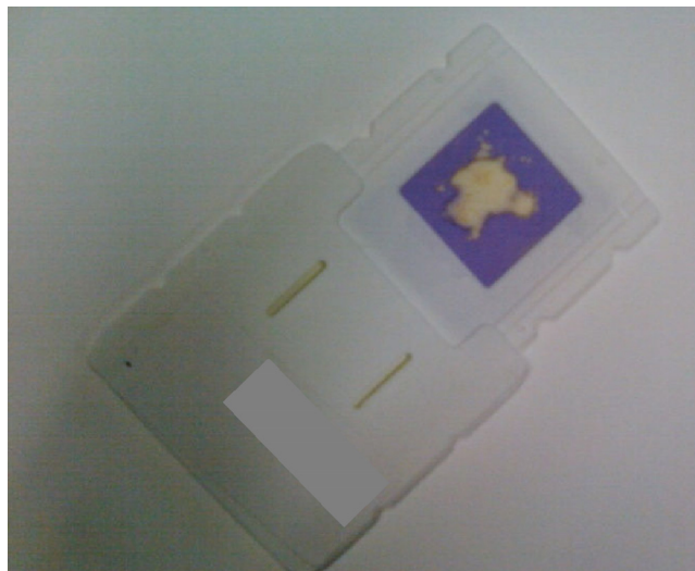
FIG. 2. Whatman indicating FTA elute cartridge upon application.
